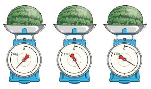
Always look carefully at how the numbers on the scales increase when reading a measurement.
